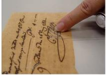
Cover with a piece of inert plastic foil, apply gentle pressure for 30s
