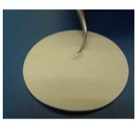
Remove excess of solvent by blotting on filter paper
