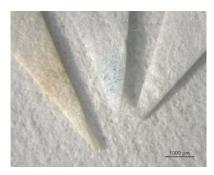
Check the filter paper under a microscope or magnifier. Migrated pigments / dyes can be easily detected
