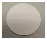
Remove the filter paper from the object and place it on a white support (filter paper)
